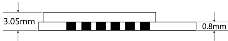
Figure -4. Module Size - shieldingcase (Side View)
